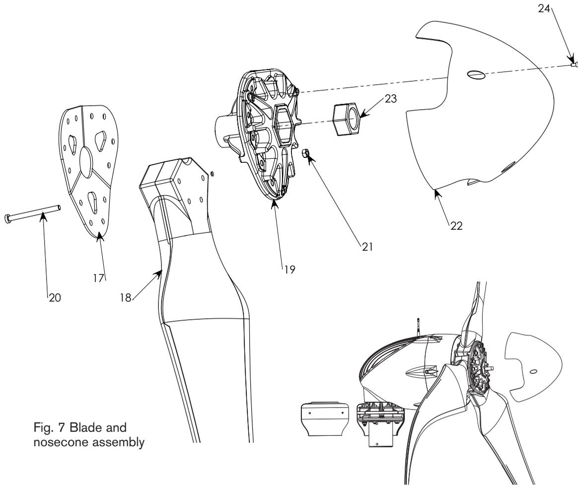
Fig. 7 Blade and nosecone assembly
