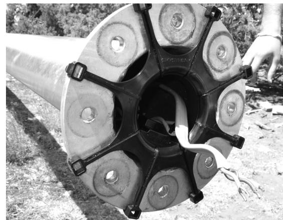
**IMPORTANT:** Install the Skylevel “spider” on the tower top prior to connecting the power wires to Skystream yaw. The wires must pass through center of “spider” as shown in accompanying photograph.
