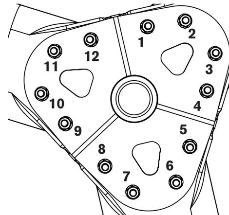
Blade bolt tightening sequence
