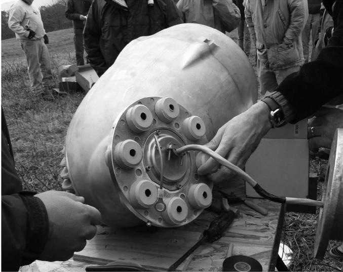
Fig. 4 Placing vibration isolators
