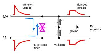
Inside the PowerTarom there are electronic components (varistors and suppressor diods) to limit the energy of transient spikes. These elements normally absorb some limited energy and convert them into heat. If the power is too big even these elements will be destroyed by overheating.
