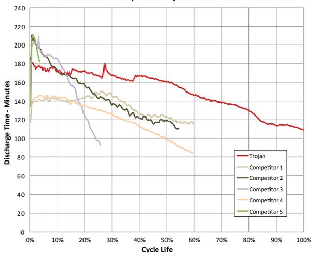
Trojan Deep-Cycle AGM Cycle Life versus Depth of Discharge
