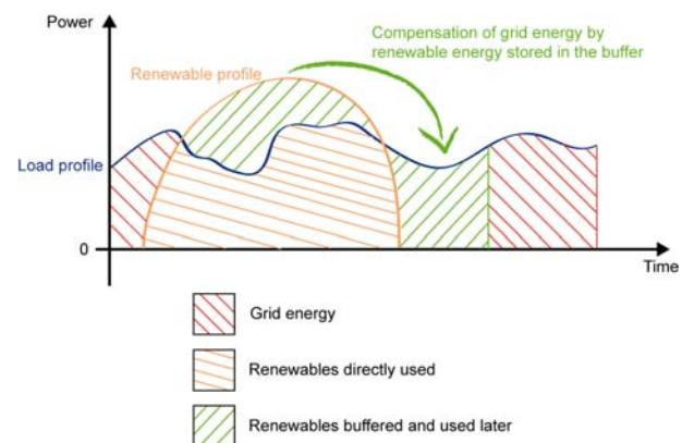
(Figure 4) Load profile with renewable energy buffered
