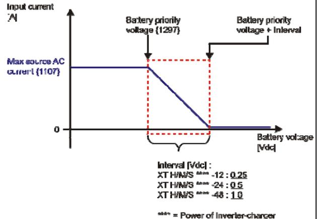
(Figure 4) Graph of Solar priority function. (Current taken on the AC source depending on the battery(ies))
