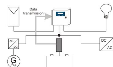
⇒ The controller transmit system parameters via power line. These parameters can be evaluated at each point of the grid with additional receivers. By this there are the following extension possibilities:
