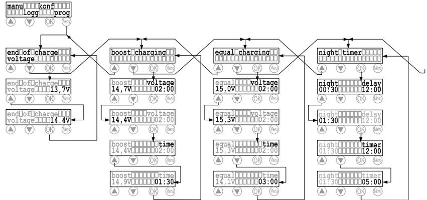
**Tip:** If you want to make sure that you have programmed correctly, exclusively press OK and move through all Boost submenus.
