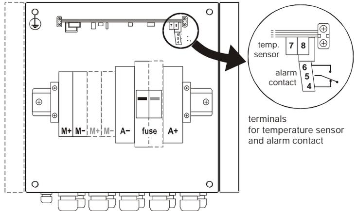
Connect loads that must not be disconnected by the controller (e.g. emergency light, radio link) directly to the battery! Increased risk of discharge no longer controlled by the system controller! Secure these loads by installation of safety fuses.
